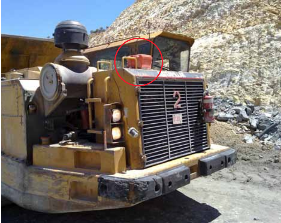
The orange box contains the datalogger, tilt sensors and 3D accelerometer. The radar speed sensor is sitting on the side of the engine down near the lights.
