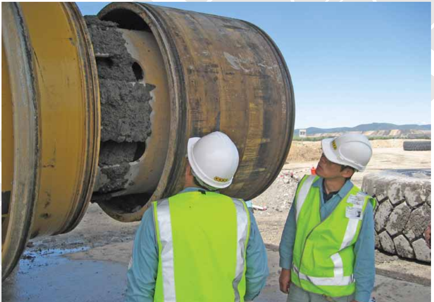
Topy engineers inspecting the condition of Smart Change and Super Strength Wheel components after prolonged service life.
