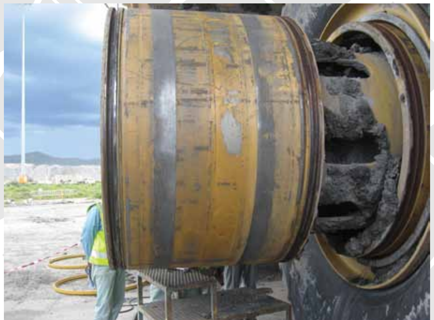
Topy's new Super Strength wheel provides up to 10 times the life of conventional rims.
